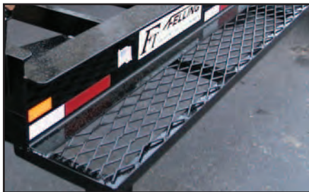
Catwalk in Front and Rear of Fender Providing Side Steps
